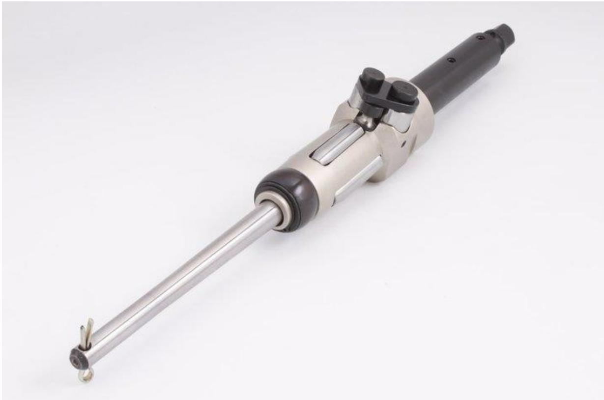
Both the tube and the beading expander should be totally clean and free of any protective rust inhibitors from the tube manufacturer. The presence of any such material will prevent the expander rolls from having the traction needed to develop the force needed to feed the beading roll against the tube end to form the bead.
