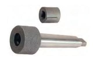
Use - Mandrel drives serve the purpose of adapting tube expander mandrels to existing air or electric drills. Loosening the knurled nut, releases the square insert type of socket for the introduction of another size of insert to couple to other size of mandrel square.
